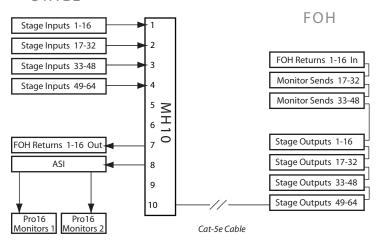
This 64x48 digital snake uses one MH10 Merger Hub. Input and output modules at the FOH position are connected serially. The ASI (connected to port 8) translates Pro64 data for use with Pro16 monitoring devices.
